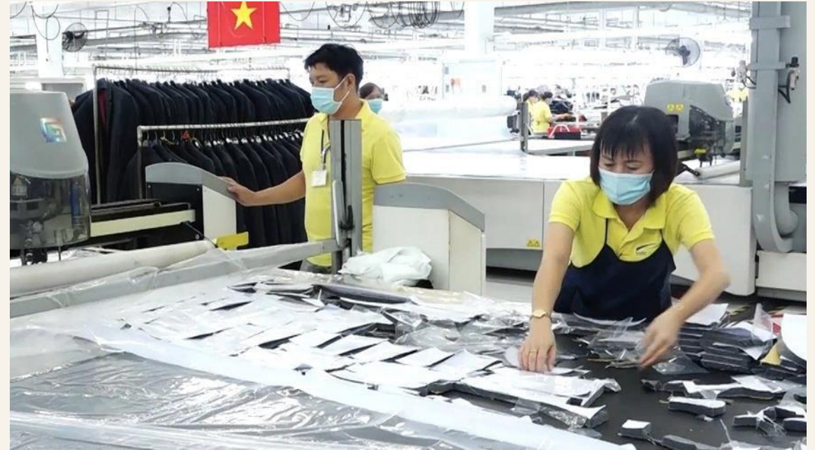
Spreading and marking on the cutting floor
